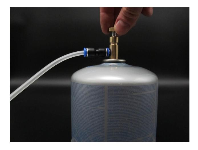
Turn the gas valve control knob clockwise, slowly until you hear small amount of gas coming out of the burner! Counterclockwise will shut down the gas!
