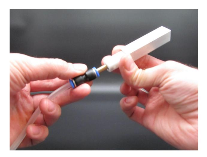
Plug the other end of the silicone hose directly to the burner side! In order to remove the burner, you must press the ring button in the push-lock fitting and by holding it you remove the burner!
