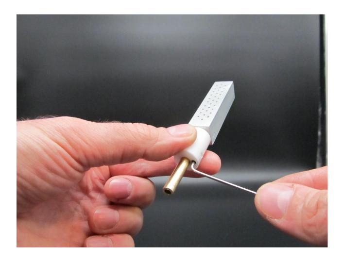
To regulate flame color (Air-fuel), you would need allen key 1.5mm! Turn the set screw on the white Teflon handle, as shown in the photo, clockwise to get yellow flame, and counterclockwise for more blue flame. Optimal flame for this burner, that have maximum height, will have blue color on the bottom and yellow on the top!
