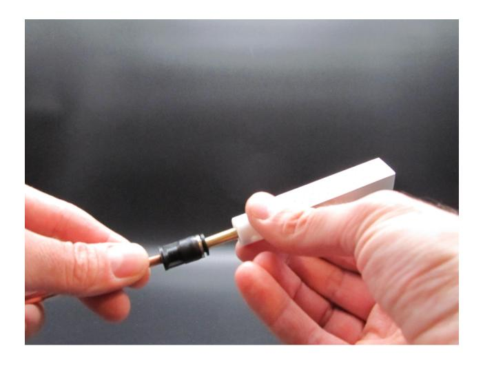
Plug the other end of the copper pipe directly to the burner side!
