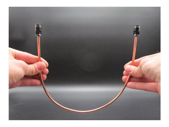
Since the copper pipe is bend inside the package, you have to shape it in a way to fit your steam engine and also to connect it to the gas tank valve!
