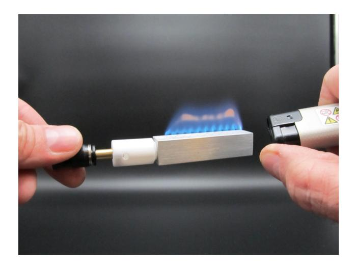
Light up the burner and get low flame at first, by slowly controling gas valve knob. Then place the burner inside your steam engine burning chamber and slowly turn the gas valve knob to get desired firepower. Be careful to not burn your hands!
