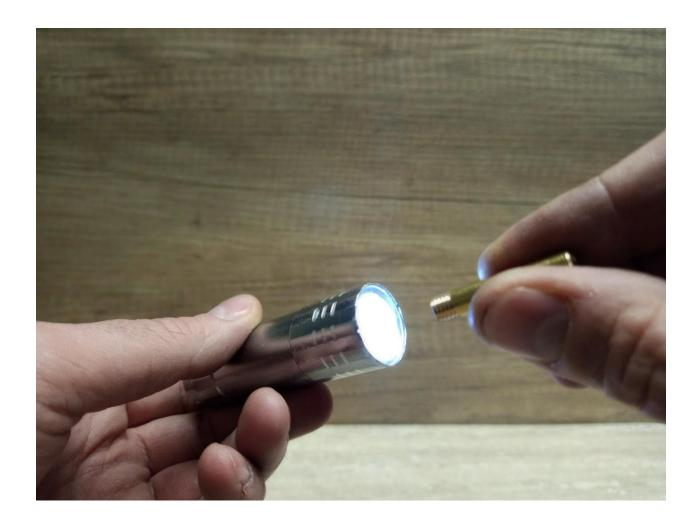
Point the gas jet thread to flashlight and look trough the jet. You should see a tiny clear hole. If you cant see the light trough the tiny hole, jet must be cleaned.
