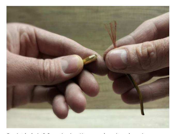
Gas jet hole is 0.2mm in size. You can clean it up by using compressed air, mouth blowing (if its not clogged too much), or you can find some old cable as shown in the photo above, trim the cable and you will find many tiny wires that are usuly tin enough for cleaning the jet hole! If the jet hole is clear, put it back inside the burner and tight it up well, and test the burner it should work fine. If necessary adjust air fuel ratio again.
