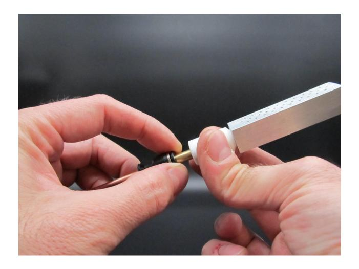
In order to remove the burner, you must press the ring button in the push-lock fitting and by holding it you remove the burner!
