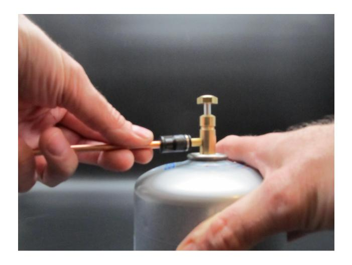
Plug the one end of the copper pipe directly to the gas valve!
